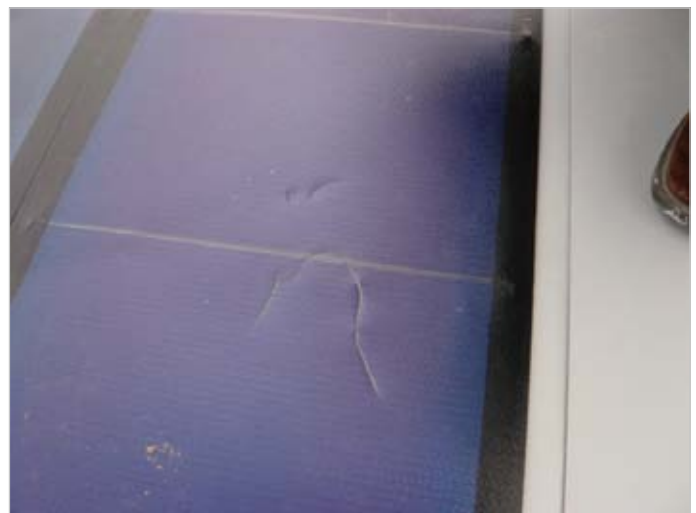
Fig. 1: Stepping onto the TF Membrane Professional can result in damage.
